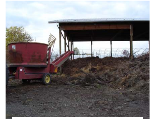
Tub grinder reduces particle size of organic matter to facilitate composting.
